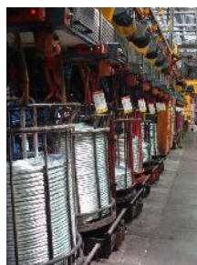
Above: The recently installed wire fluid bed heat treatment furnace which replaced lead baths.
