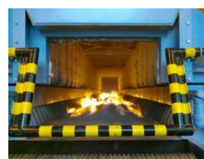
Above: The recently installed wire fluid bed heat treatment furnace which replaced lead baths.
